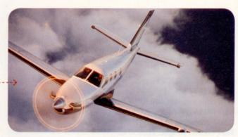
Daher-Socata officials position the TBM 850 as having jet speeds (320 KTAS) with the lower operating costs typical of a turboprop. It is claimed to climb to 31,000 feet in 20 minutes and fly 1,400 nm at economy settings, yet use a 2,100-foot runway—shorter when propeller reverse is applied. It comes standard with Garmin G1000 integrated avionics.
