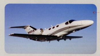
The Mustang is the lightest of the new generation of small, single-pilot very light jets. But Cessna would rather you call it a light-light jet. Either way, the Mustang has been a success, with more than 200 deliveries since its debut in 2007. It features the Garmin G1000 avionics suite, a max operating altitude of 41,000 feet, and a side-facing, non-belted lavatory seat.
