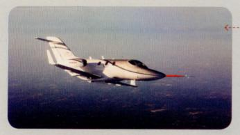
Honda has taken a patient, innovative approach to its first foray into the GA marketplace with a twinjet that uses over-wing engine pylons, composite materials, and an engine developed with General Electric. The first HondaJet flew in 2003, and conforming prototypes have turned in exceptional performance in speed and efficiency at altitudes up to 43,000 feet.
