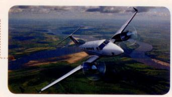
The new King Air 250 has a Rockwell Collins Pro Line 21 avionics suite plus 850-shp Pratt & Whitney PT6A-52 engines. Maximum cruise is 310 knots. The basic operating weight compared to the previous B200GT model is 355 pounds greater. Useful load decreased from 4,165 pounds for the now-replaced B200GT to 3,810 pounds for the King Air 250.
