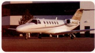
True to Cessna's Citation marketing strategy, the CJ2+ represents an incremental jump in performance over the now-out-of-production CJ1+. The CJ2+, with its more powerful engines, breaks the 400-knot cruise mark, is 30 knots faster than the CJ1+, and can fly 300 nautical miles farther. The CJ2+ cabin is three feet longer than that of the CJ1+.
