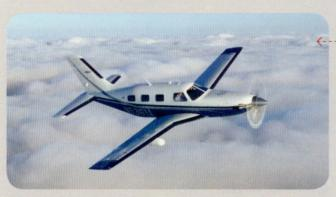
The turboprop Piper Meridian has become a mainstay of the Piper fleet despite competition from VLJs and turbocharged pistons. The six-seat Meridian with its 500-horsepower PT6A-42A can reach 30,000 feet (limited to 28,000 in RVSM airspace), several thousand feet above high-performance pistons. The Meridian is equipped with the Garmin G1000 avionics suite.
