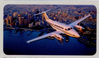
This is the top-of-the-line King Air, and it uses Rockwell Collins Pro Line 21 avionics. It is powered by two 1,050-shp Pratt & Whitney PT6A-60A engines and promises a typical high-speed cruise of 312 knots. If you need extended range or a high-performance special-mission aircraft, the King Air 350iER is available for \$8.06 million, with a promised typical high-speed cruise of 303 knots.
