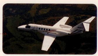
The CJ4 is the top of the CJ line and the latest of the CJs to be certified. Deliveries began in 2010. Thanks to its 3,400-lb-thrust engines and swept wings, the CJ4 surpasses the 417-knot maxcruise-speed barrier. Single-point refueling is standard, as is a new, lighter lithium-ion battery, a new entry-door design, four-panel spoilers, and a ground-spoiler feature.
