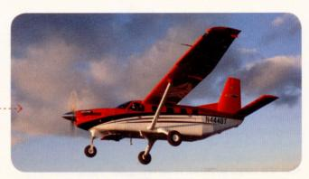
The Quest Kodiak was developed specifically for missionary operations to unimproved runways. The utility aircraft has a Garmin G1000 glass cockpit and can cover more than 1,000 nm with IFR fuel reserves at cruise speeds up to 183 KTAS. It is powered by a Pratt & Whitney PT6A-34 and can be adapted to a wide variety of cargo and passenger configurations.
