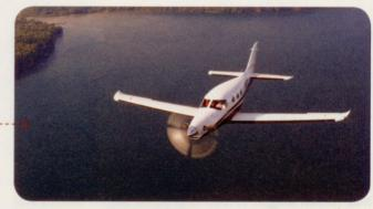
The all-composite Kestrel is meant to fit into the single-engine turboprop marketplace somewhere between the TBM 850 and the Pilatus PC–12. With its six to eight seats, a 325-knot cruise, and target price of \$3 million, CEO Alan Klapmeier says he expects to sell and produce 75 new airplanes a year.
