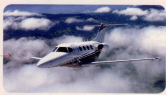
With a max cruise speed of 454 knots, the Beechcraft Premier 1A is the fastest of the single-pilot jets. It features swept wings, a composite-construction fuselage, and Rockwell Collins Pro Line 21 avionics. The airplane's comparatively large cabin dimensions and a lift-dump system that uses a maximum flap deflection to assist in braking after touchdown are notable.
