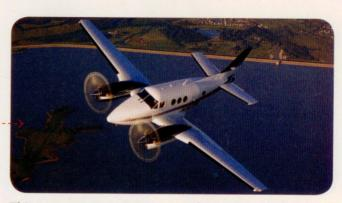
This newest variant of the very popular C90 series includes a Rockwell Collins Pro Line 21 avionics suite and 750-shp Pratt & Whitney PT6A-135A engines, flat-rated to 550 shp. The result is an airplane with a max cruise speed of 272 knots and a max range as far as 1,236 nm. The big news in this latest model is a 300-pound increase in payload with full fuel.
