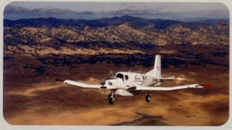
This all-metal, fixed-gear utility plane built in New Zealand by Pacific Aerospace Ltd. was originally developed to haul skydivers but also is marketed as a utility aircraft. It was certified in the United States in 2004 and carries a single pilot and up to nine passengers. The aircraft has a range of 582 nm.
