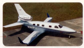
Piper Aircraft has rebranded the PiperJet "Altaire" and made design changes, including a larger cabin, longer wing, and shortened vertical tail. The PiperJet logged more than 400 flight-test hours and pioneered an automated trim system designed to adjust for power changes in the single tail-mounted engine. Customer deliveries are scheduled to begin in 2014.
