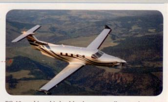
PC–12s are big-cabin load-haulers *par excellence*, and most are ordered with a stylish seven-seat interior designed by BMW DesignWorks USA. The airplane features a single 1,200-shp Pratt & Whitney PT6A-67P engine, a forward air stair door, and a huge aft cargo door that is remotely operated.
