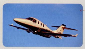
The D-JET is among the easiest to operate of the VLJ designs, with its single turbofan engine and 25,000-foot max operating altitude. Its 5,690-pound max ramp weight also makes it the lightest of the light jets. The cockpit is centered around the three-screen Garmin G1000 avionics suite. It has been in development since 2007, and certification is expected in late 2012.
