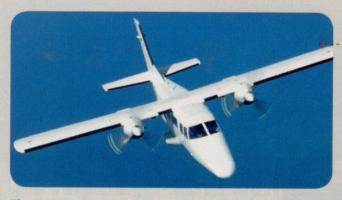
The A-Viator is a multipurpose, high-wing turboprop twin with entry-level simplicity. A large, unpressurized cabin can be configured for executive or charter use. The A-Viator is derived from a long line of Italian-built designs, and as such closely resembles the Partenavia series of light piston twins and turboprop twins.
