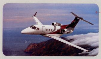
The Brazilian-built Phenom 300 is the Phenom 100's bigger brother. The 300 features slightly swept wings and 440-knot max cruise speeds, and it shares the 100's three-screen Garmin G1000-based Prodigy avionics suite. The popular Phenom 300 is a direct competitor of Cessna's CJ4—which has virtually identical performance specifications, but at about \$1 million less.
